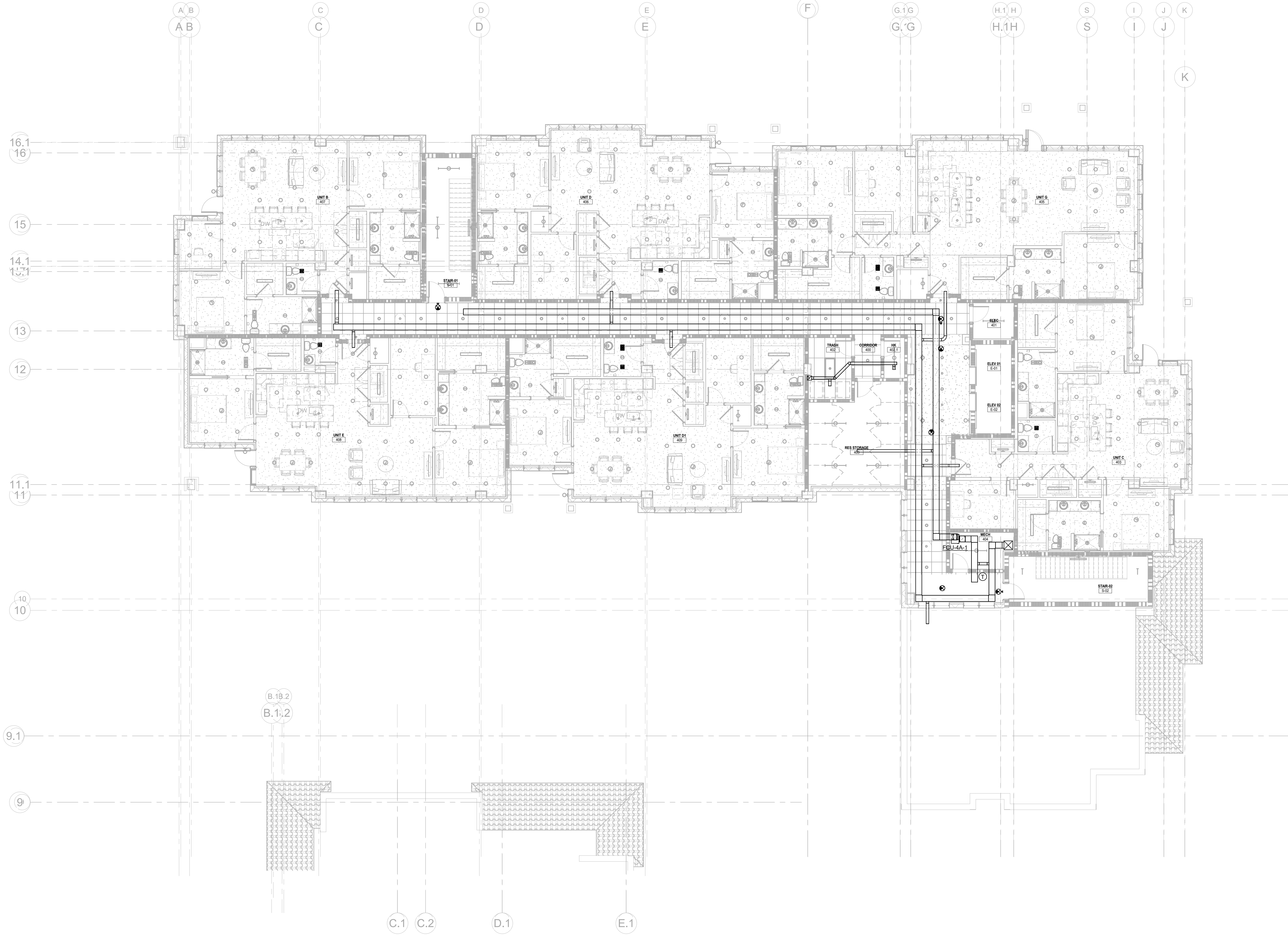
1 MECHANICAL PLAN - FOURTH FLOOR - AREA A M-144-A 1/8" = 1'-0"
