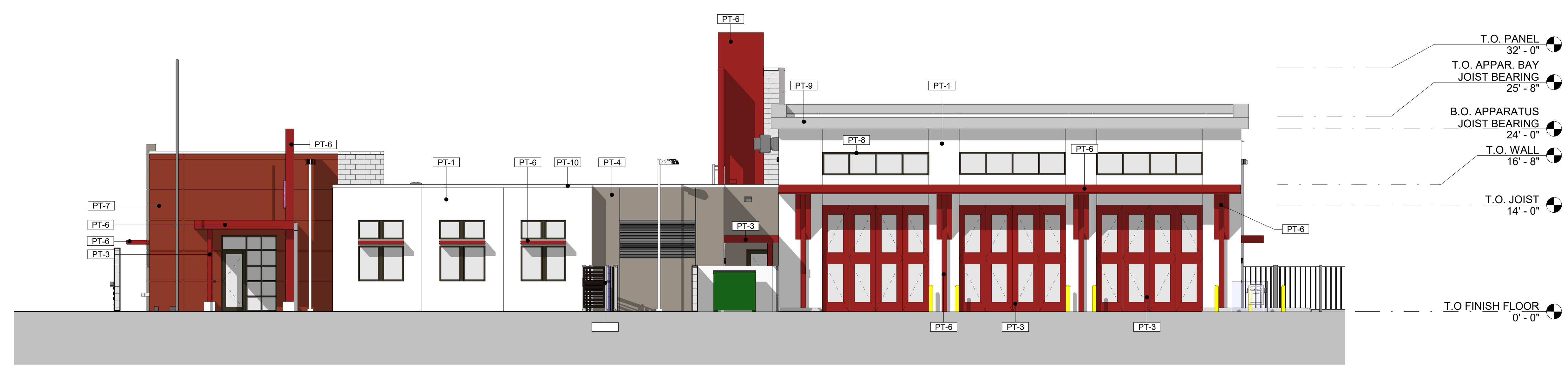
2 A3.04 EXTERIOR ELEVATION- WEST (MATERIALS) 1/8" = 1'-0"
